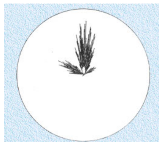
A typical picture of a pattern of a lobe switching radar on a DBM-1 shows that the pulses are of different lengths but do not appear to be arranged in groups.
